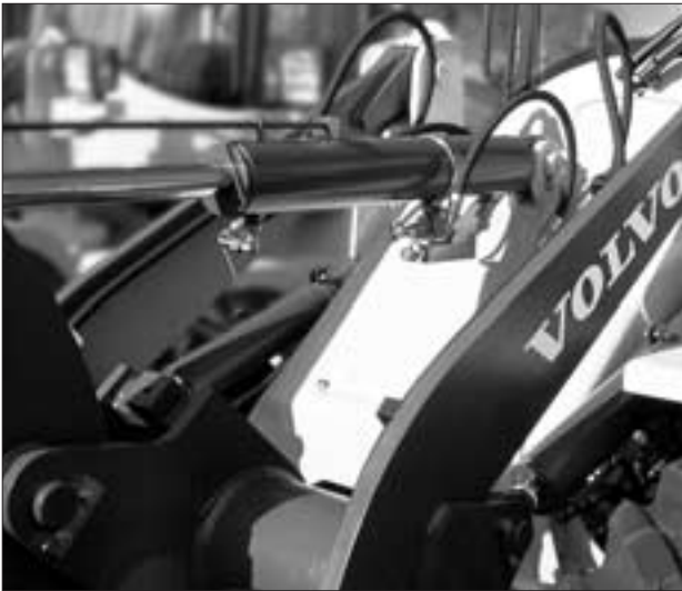
Tilt Cylinder Dump Control Valve to be used with buckets with grapples
